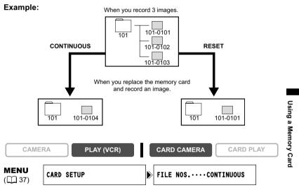
To change the setting, open the menu and select [CARD SETUP]. Select [FILE NOS.], set it to [RESET] and close the menu.
