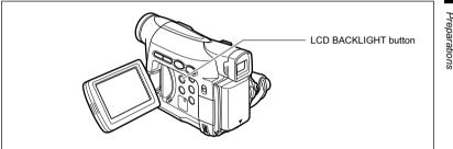
You can switch the brightness of the LCD screen between normal and bright by pressing the LCD BACKLIGHT button. This is useful for outdoor recordings.
