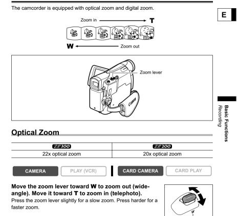
O You can also use the **T** and **W** buttons on the wireless controller. However, you cannot control the zoom speed.
