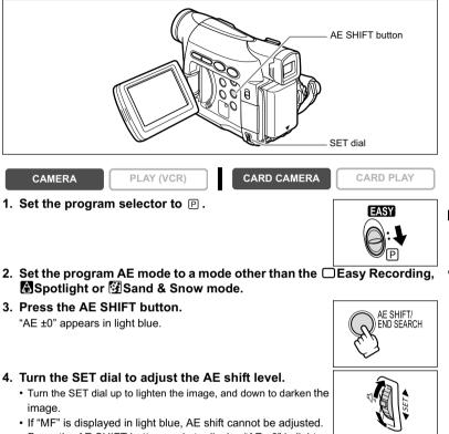
If "MF" is displayed in light blue, AE shift cannot be adjusted Press the AE SHIFT button again to display "AE ±0" in light blue.
